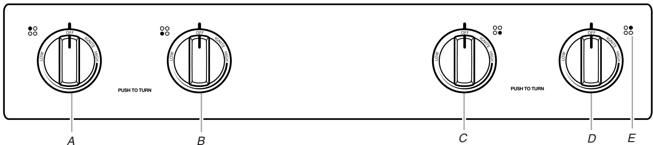
A. Left rear burner control B. Left front burner control (Power™ burner on some models)
